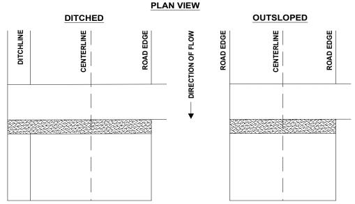
It should be sloped to drain with a relief ditch through the down slope edge of the road. The trench shall be behind the berm for approaching traffic.
