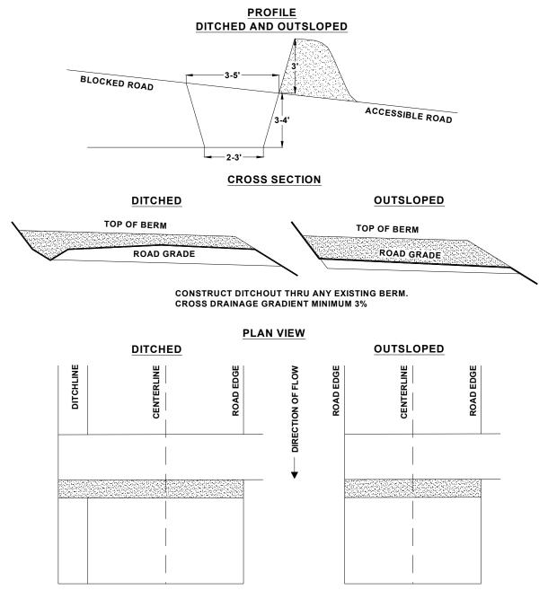
It should be sloped to drain with a relief ditch through the down slope edge of the road. The trench shall be behind the berm for approaching traffic.
