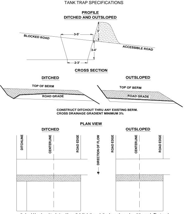
It should be sloped to drain with a relief ditch through the down slope edge of the road. The trench shall be behind the berm for approaching traffic.
