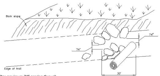
Filter maximum 74" spacing through path entrance and exit. 6'- 8' curve radius through filter. Overall length of filter should be 30'. Boulders used as blocking material should be buried 1/3 of original height.
