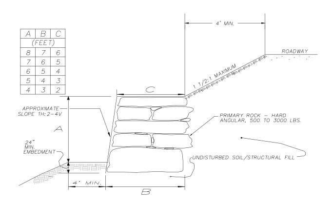
ALL ROCKS TO BE SOUND, UNWEATHERED ANGULAR ROCK. PRIMARY ROCK SHALL BE 500—3000 LBS AND SHALL NOT BE MOVABLE WITH A PRY BAR. ROCKS SHALL BE TIGHTLY NESTED (LOCKED TOGETHER) WITH ALTERNATING JOINTS AND WITH LARGER ROCKS AT BOTTOM. RIPRAP SHALL BE FREE DRAINING THROUGH SMALLER RIPRAP FILLED VOIDS. EACH ROCK SHOULD REST ON AT LEAST TWO ROCKS BELOW IT.
